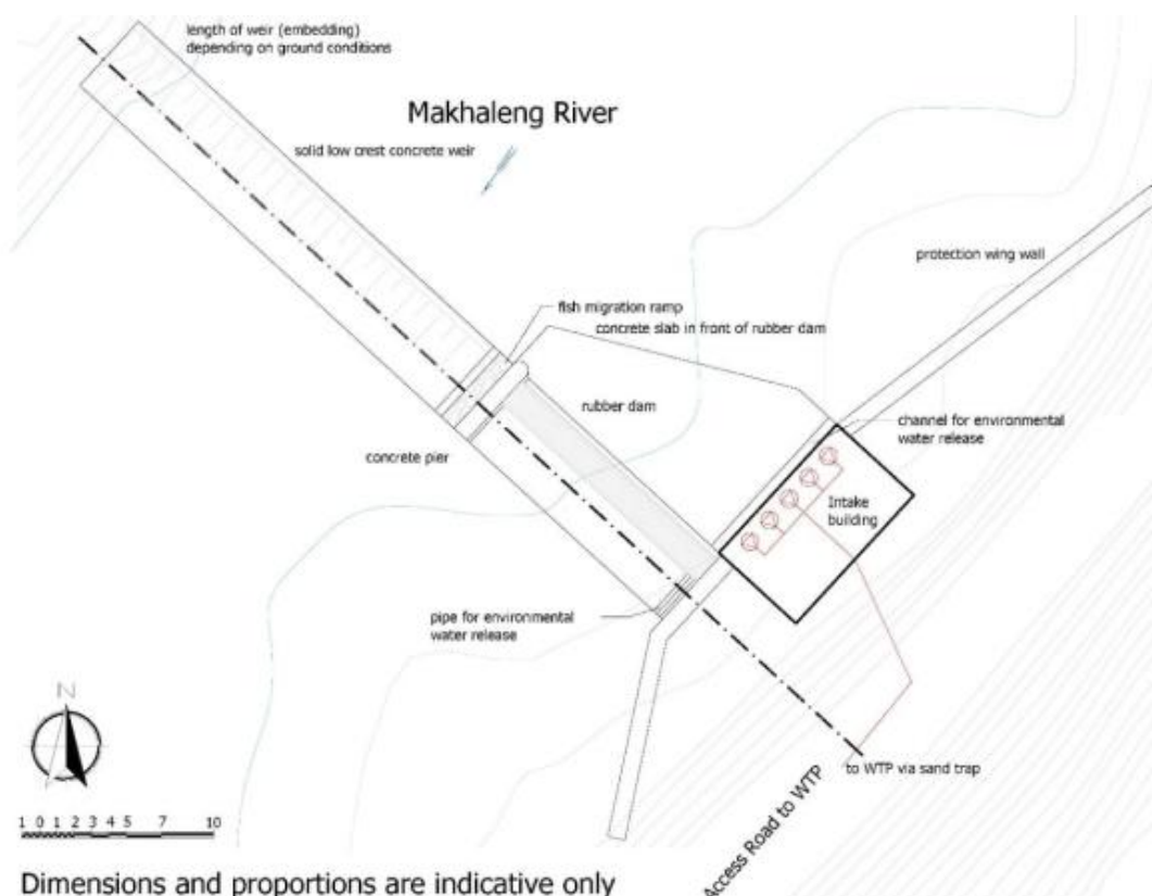
Figure 12 Plan View of the Proposed Weir and Intake (P&P; July 2018)
